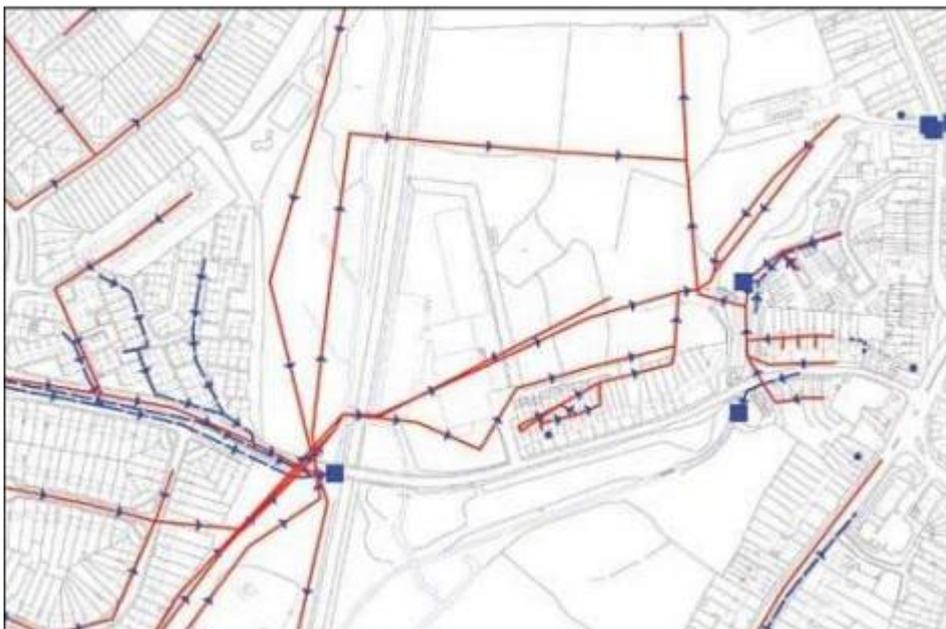
***A typical drainage plan showing the location and direction of surface and foul water sewerage systems. Surface sewers are marked in blue and foul sewers in red Picture courtesy of Severn Trent Water***
