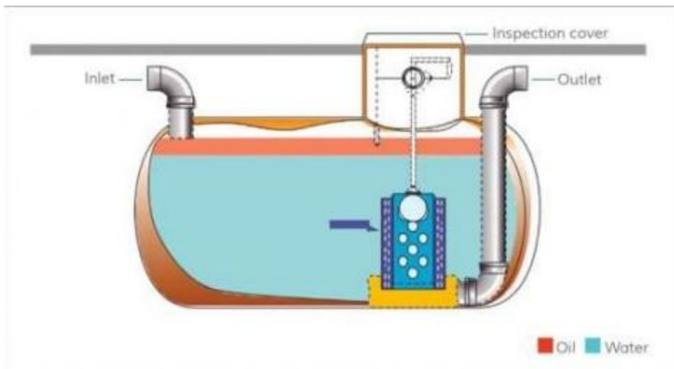
**A single-Single chamber oil separator showing oil or fuel floating on top of water**
